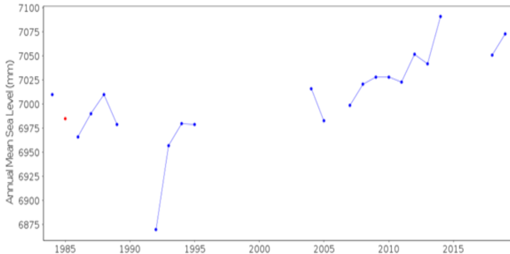
Figure 2: Tide gauge information at Ilfracombe indicates a RSL in the order of 3mm per annum. Consequently, the extent of saltmarsh is reducing within the estuary due to coastal squeeze, against the flood defence that was the former railway line circumscribing the estuary. © https://www.ntsfl.org/products/sea-level-trend-charts?name=Ilfracombe
